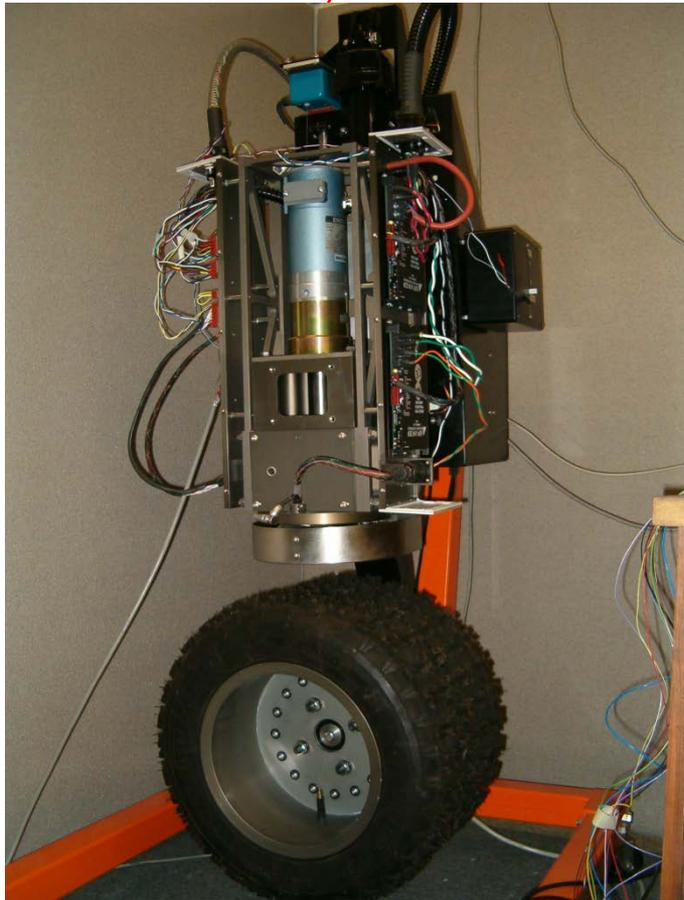
The Smartwheel Networked Control Testbed Demonstration System
