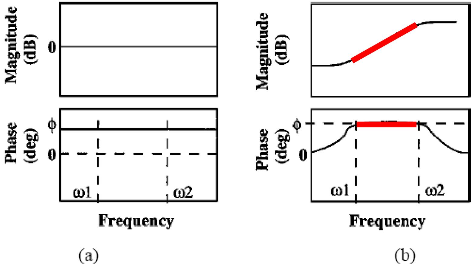
Fig. 10. Frequency response. (a) Ideal phaser. (b) Approximation.
