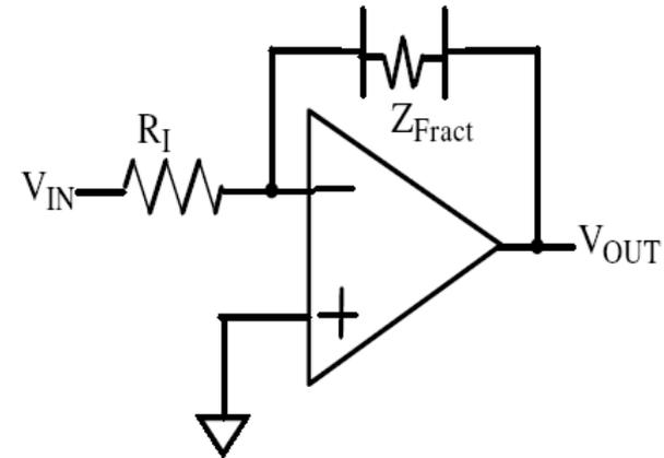
Fig. 2. Schematic for a fractional order integrator.  $Z_F$  represents the Fractor™ element. The schematic symbol for the Fractor™ was designed to give the impression of a generalized Warburg impedance; a mixture of resistive and capacitive characteristics.
