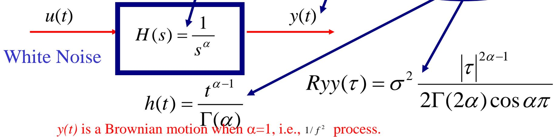
$1/f^{2\alpha}$  noise (signal) generation via fractional dynamic system
