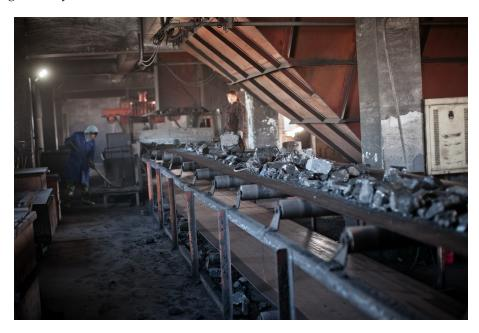
Figure 1. Manual separation of coal and gangue.
