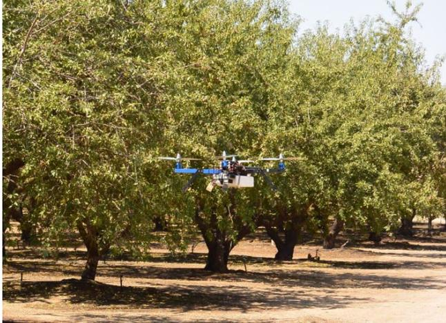
**FIGURE 2.** THE UAV-BASED REMOTE SENSING PLATFORM INCLUDING A QUADCOPTER, A NIR CAMERA AND A RGB CAMERA, CREDITS TO LARRY BURROW.
