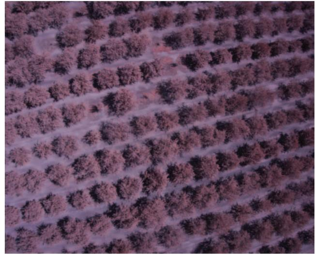
Fig. 3: The wavelength dependence on BRDF can be visually seen by the change in color of the trees from the right to the left of this image taken with a G-B-NIR modified camera (ELPH110).
