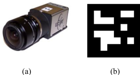
Fig. 3. Tracking hardware: (a) Power-over-Ethernet camera; (b) tracking marker pattern.
