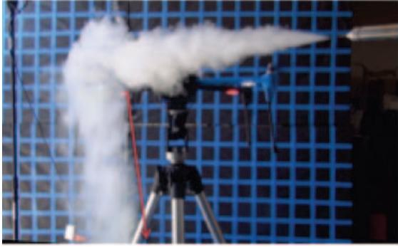
Fig. 4. Cylindrical downwash produced by propeller outtake
