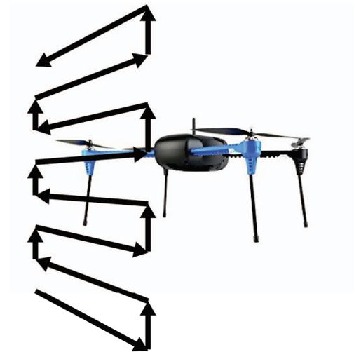
Fig. 2. Illustration of lawn mower pathway performed with a smoke wand
