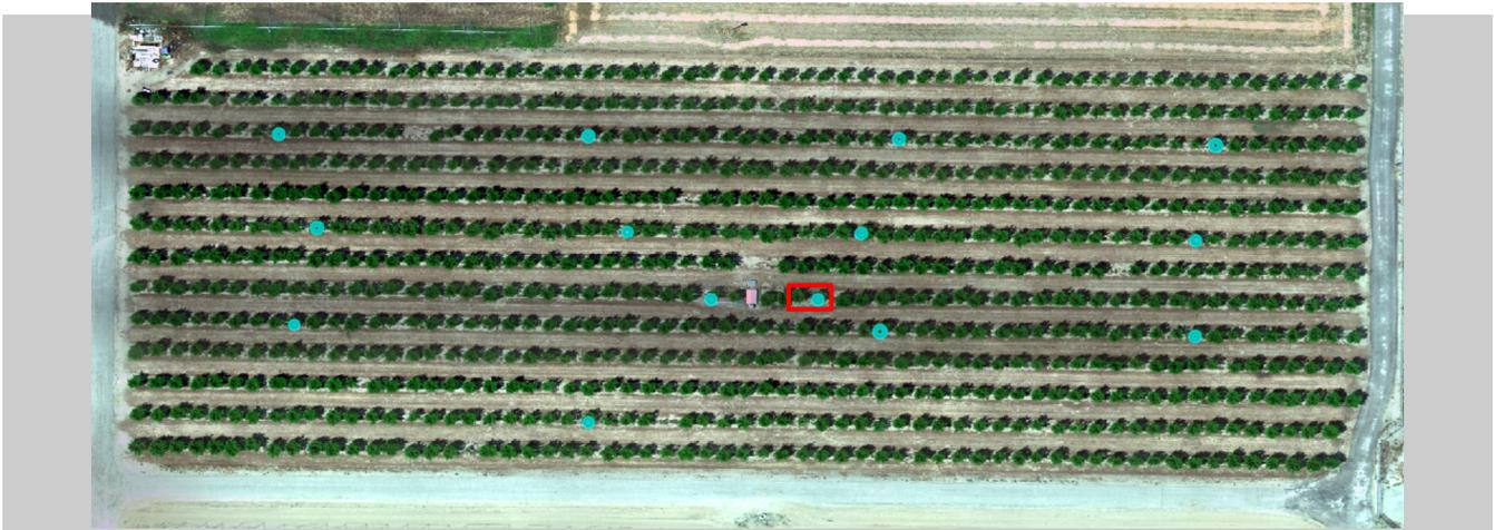
Fig. 1. The pomegranate field at the USDA-ARS (36.594°N, 119.512°W). The weighing lysimeter is located in the center of the pomegranate field, marked as a red box. The blue marks are where the 14 IRT sensors were installed.
