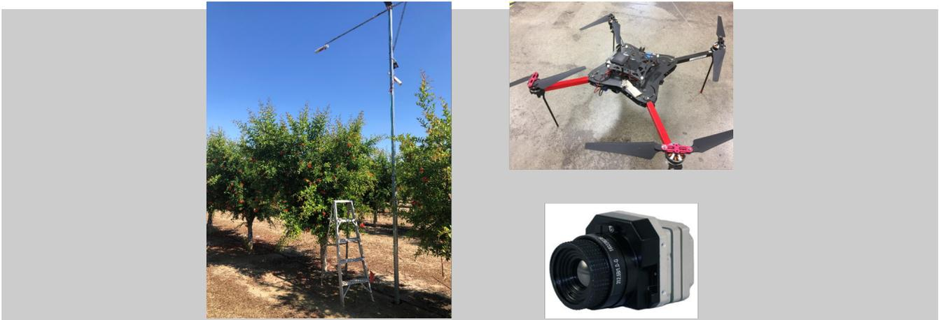
Fig. 2. The IRT sensors were mounted on a cross arm attached to a metal pole 4.5 m above the soil surface, with a FOV of 20°. A quadcopter and a thermal camera were used to collect high-resolution thermal images at the height of 60 m.
