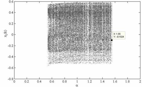
Fig. 1. Bifurcation diagram of generalized discrete fractional Henon chaotic system
