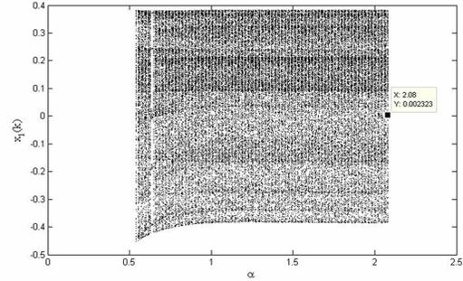
Fig.3. Bifurcation diagram of discrete fractional Henon chaotic system
