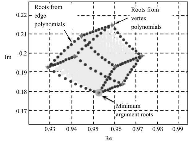
Fig. 4. Root region of expanded degree integer order interval polynomial  $\Delta^{10}(v) = [2.1 \ 2.6]v^{21} + [1.2 \ 1.7]v^8 + [0.7 \ 1.3]$  in the first Riemann sheet. Roots from edge polynomials and roots from vertex polynomials of hyper-rectangle  $A$  are indicated by blue dots and red asterisks, respectively.
