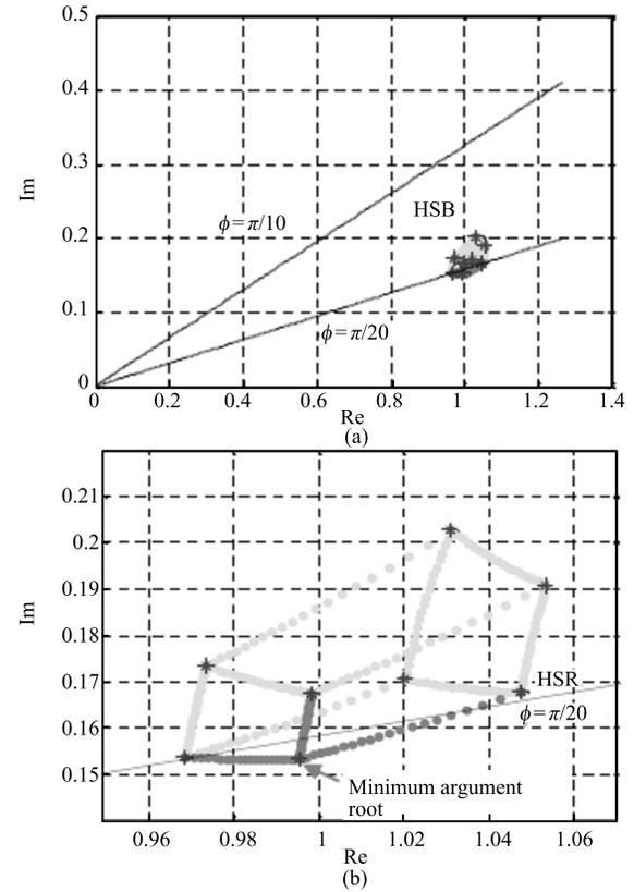
Fig. 6. Root placement for Example 1 ((a) Roots of vertex and edge polynomials; (b) Close view of minimum argument vertex and connected edge polynomials.)
