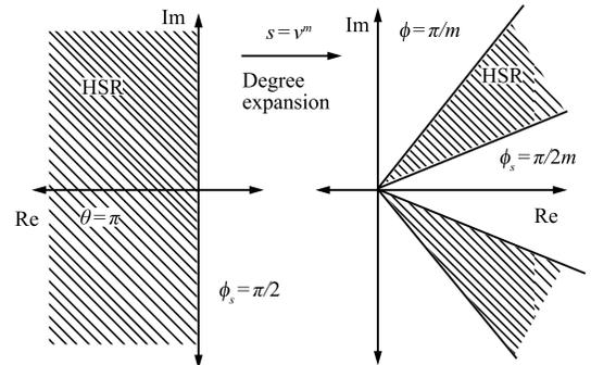
Fig. 1. Hurwitz stability region of fractional order characteristic polynomials under  $s = v^m$  mapping<sup>[4]</sup>.
