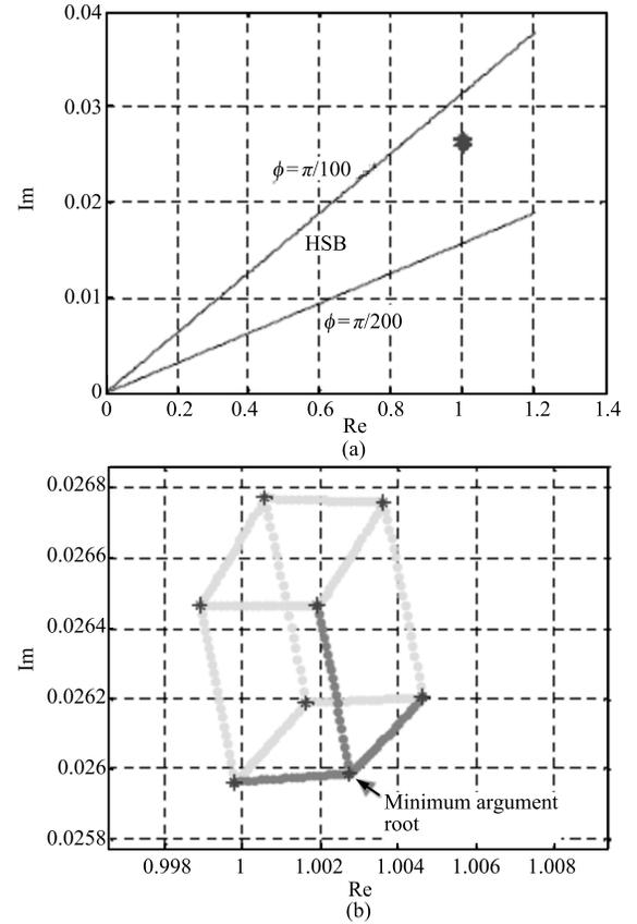
Fig. 8. Root placement for Example 2 ((a) Roots of vertex and edge polynomials; (b) Close view of minimum argument vertex and connected edge polynomials.)
