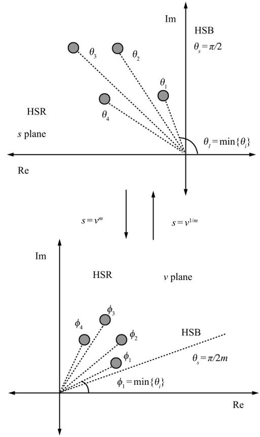
Fig. 2. Argument and magnitude relations are conformal under power mappings (Root placements in  $s$  and  $v$  planes conserve argument relations).
