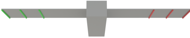
Fig. 6: Perspective view of underwing lights perpendicular with leading edge of wing.
