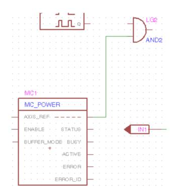
Create Signal Flow and Data Flow Connections (AND2 -> MC\_MOVE\_ABSOLUTE)
