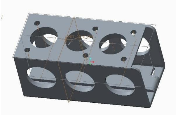
Fig. 6. A model of the battery housing, which is mounted to the base of the rotating disk
