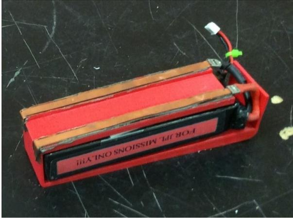
Fig. 5. The modified battery with the designed batter case
