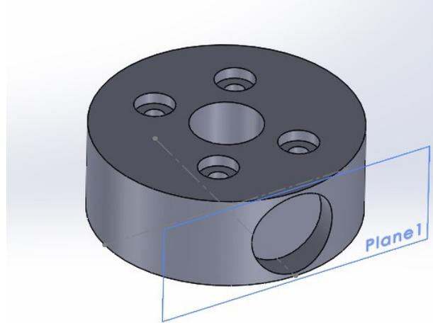
Fig. 7. The rotating attachment that allows only the battery to be rotated during battery replacement
