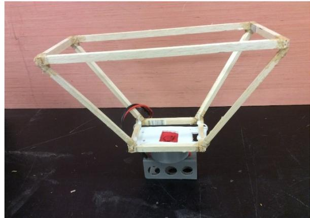
Fig. 8. The male funnel equipped with the battery housing via the rotating disk
