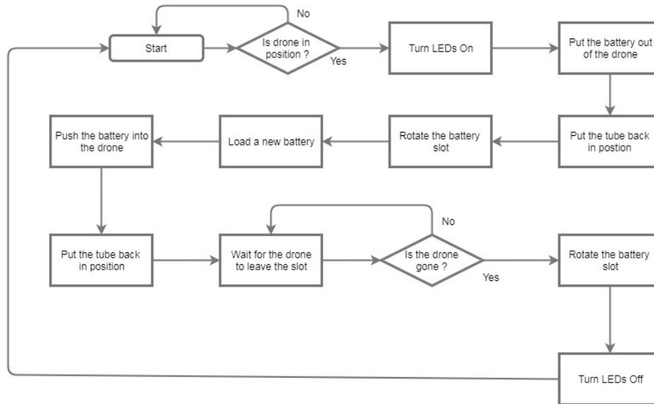
Fig. 3. The flowchart of battery swapping mechanism
