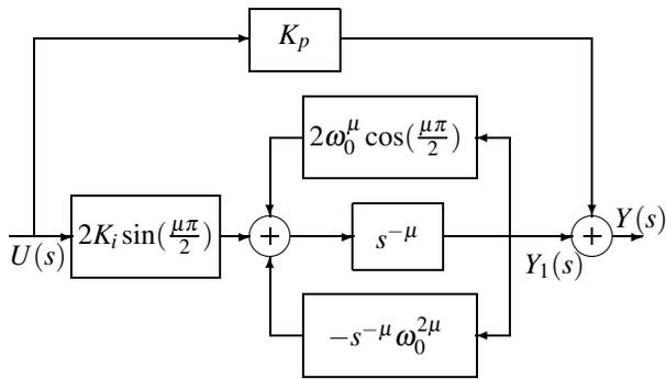
Fig. 3. Block diagram of FO-PR controller implementation
