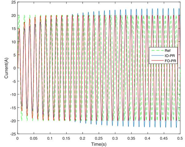
Fig. 8. Comparison of FO-PR (red line) vs. IO-PR (blue line) in the presence of frequency fluctuation. Reference signal is depicted in green dash line.
