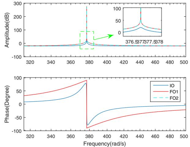
Fig. 4. Frequency responses of FO-PR and IO-PR controllers with  $\omega_0 = 2 * \pi * 60 \text{rad/s}$  and  $\omega_c = 0.1 \text{rad/s}$
