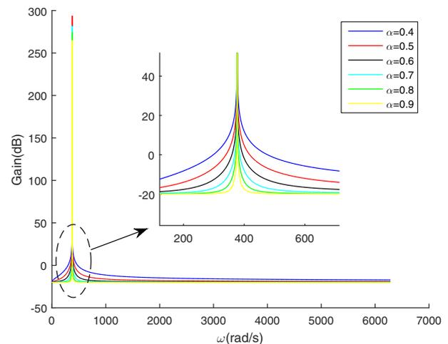
Fig. 5. Frequency responses of FO-PR controller for different values of  $\mu$  with  $\omega_0 = 2 * \pi * 60 \text{rad/s}$  and  $\omega_c = 0.1 \text{rad/s}$
