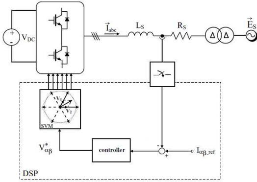
Fig. 6. Block diagrams of design example current regulator [35]
