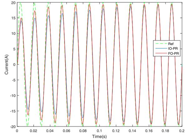
Fig. 7. Comparison of FO-PR (red line) vs. IO-PR (blue line). Reference signal is depicted in green dash line
