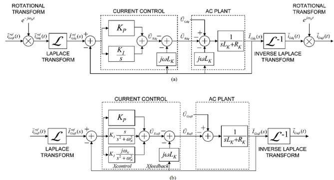
Fig. 1. (a) Synchronous frame current control loop with rotational transform operators at the input and output, (b) Stationary frame current control loop equivalent to the synchronous frame model [5]
