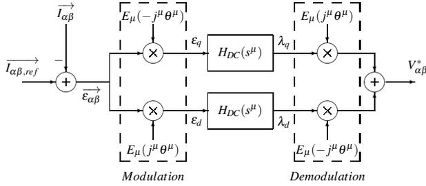
Fig. 2. Block diagram of modulation/demodulation of FO-PR controller using Mittag-Leffler function
