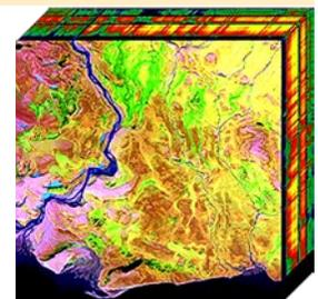
Higher cost than the other sensor types profiled here. Generates large amounts of data and requires more sophisticated methods of data analysis. Not appropriate for photogrammetric estimates of surface elevation.
