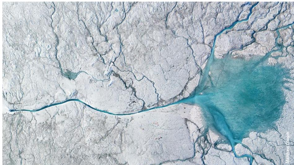
To monitor meltwater fluxes across the surface of the Greenland ice sheet, researchers generated orthomosaics like this one from digital imagery shot by a Canon point-and-shoot camera mounted on a 3D Robotics Solo drone.
