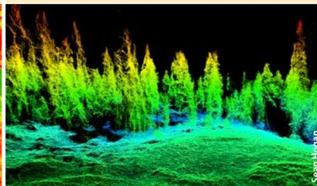
Collects elevation data but not spectral data. Generally most suitable for mapping surfaces below a vegetation canopy, because lasers have better penetration than spectral instruments. LIDAR sensors tend to be heavier than others.
