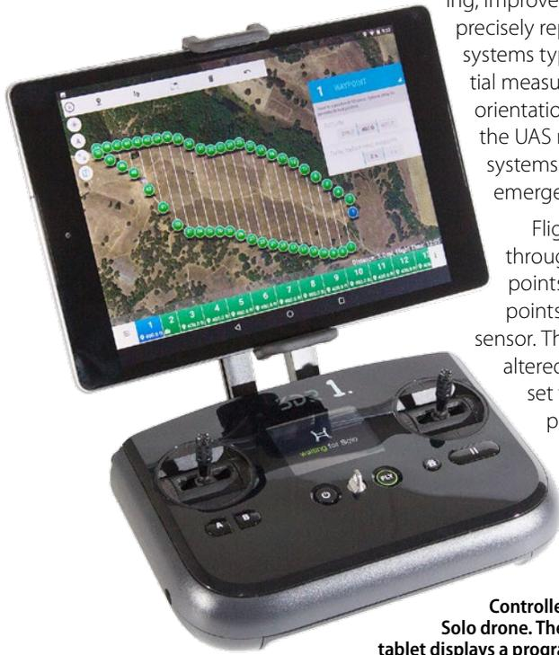
**Controller for a 3D Robotics Solo drone. The attached Android tablet displays a programmed flight plan.**
