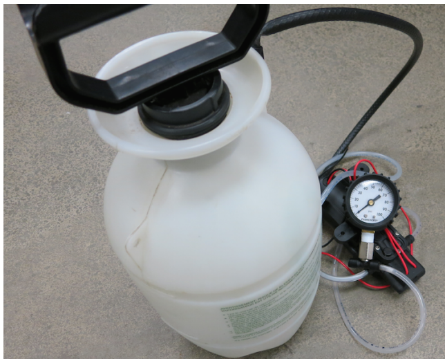
Fig. 5: Low cost and low volume sprayer for small VTOL drones
