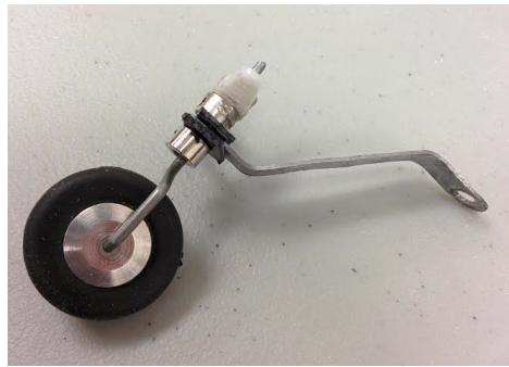
Figure 6: Rear Landing Gear Wheel, with custom steel piece
