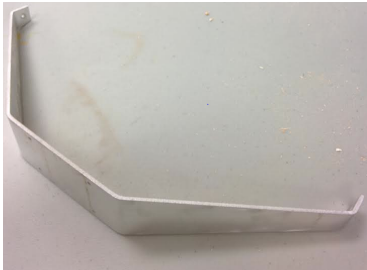
Figure 5: Landing Gear Wide-bottomed "U" Shape
