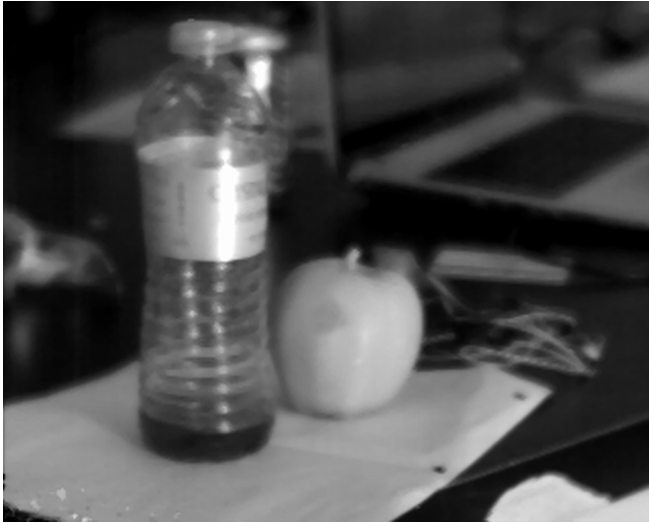
Fig. 2: Water and Bruised Apple. The bruise is imperceptible in visible light, but is visible in the SWIR spectrum.
