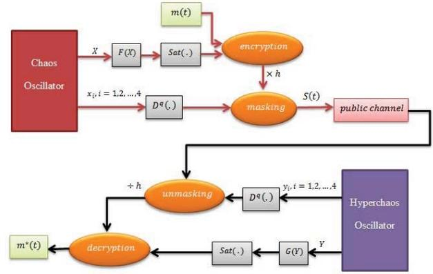
Fig. 5. The secure communication scheme based on the synchronization of FO chaotic and hyper-chaotic systems.
